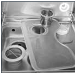
Multi filters in the wash chamber
