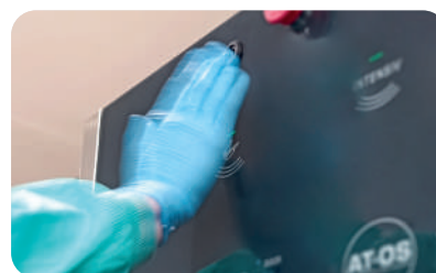
START OF THE WASHING CYCLE WITH THE SIMPLE MOTION OF THE HAND IN FRONT OF THE N.T.T PANEL
